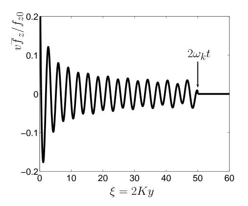
Spin polarization  $v\overline{f}_z/f_{z0}$  as a function of  $\xi = 2Ky$  calculated for the half space y > 0.
