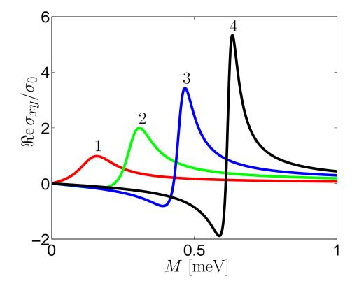
ac conductivity, Rashba model, resonances due to SOI. Parameters:  $\omega \tau = 0.5$  (1), 1 (2), 1.5 (3), and 2 (4).  $\sigma_0$  is given by  $e^2 m \alpha^2 \tau / (\pi \hbar^4)$ . In addition:  $\beta = 0$ ,  $\alpha = 10^{-9}$  eVcm,  $\tau = 1$  ps, and  $n = 10^{10}$  cm<sup>-2</sup> **Two different definitions** for the spin current (which does not enter Maxwells equations):
