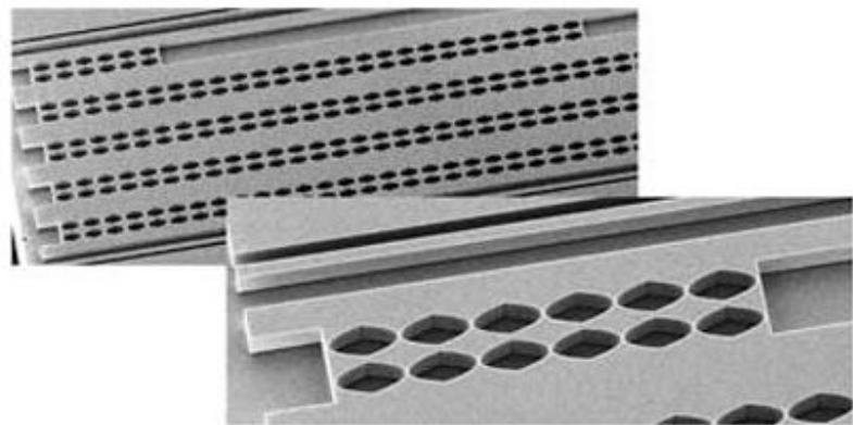
Scanning electron microscope images of silicon bilenses carefully designed to create a novel type of x-ray interferometer.
