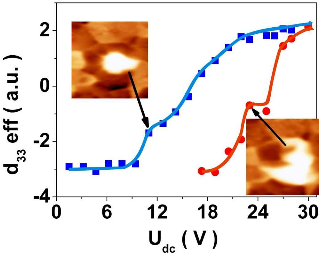
Using  $d_{33}(V)$  mapping notable kinks are observed
