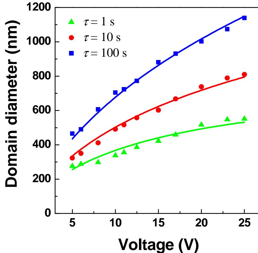
Proposed equation for the writing time and voltage of domain diameter D
