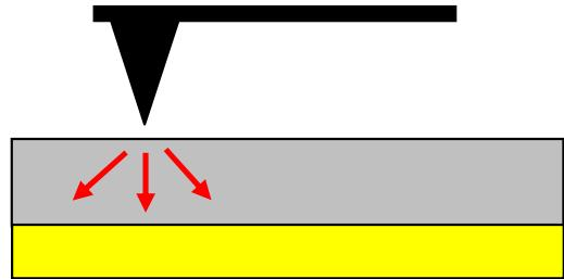
The bias is applied between tip and bottom electrode
