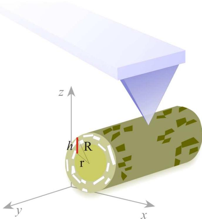
The cross-sectional distribution of the piezoresponse across and along the TGS fibers representing the TGS/PEO distribution.
