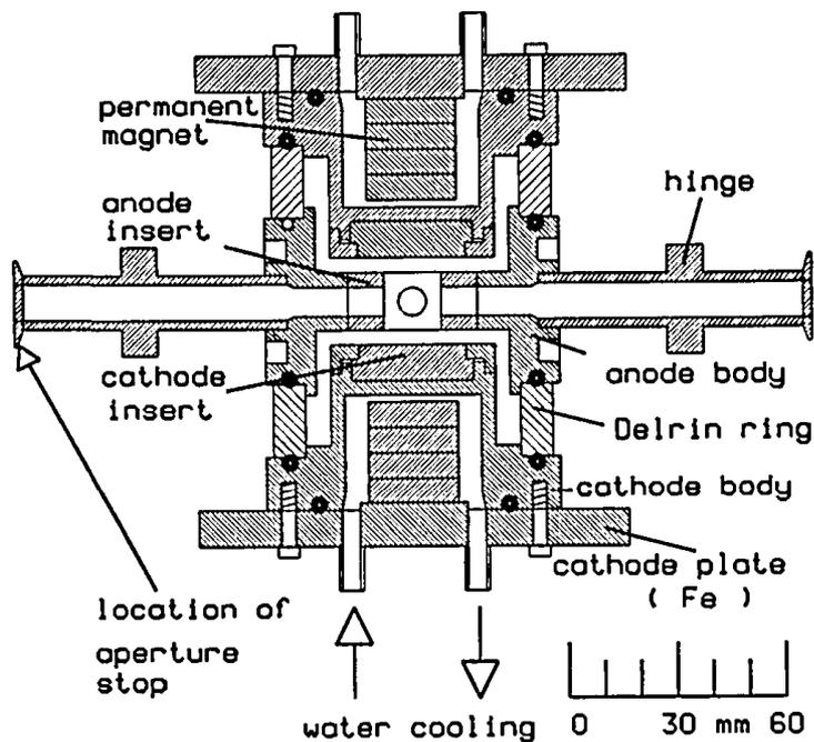
Fig. 1. Sectional drawing of the double-cathode Penning source. The two permanent magnets behind the cathodes attract each other so that the magnetic field is parallel to the electric field of the cathode falls. The anode body has four view ports at right angles for pumping, gas inlet, and observation.
