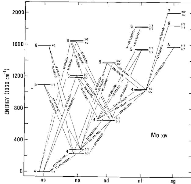
FIG. 2. Grotian diagram for Mo XIV. Wavelengths are in Å. Intensities are indicated in parentheses following the wavelengths. Wavelengths for the 4s-5p, 4s-6p, and 4p-5d transitions are those calculated from the optimized level values.
