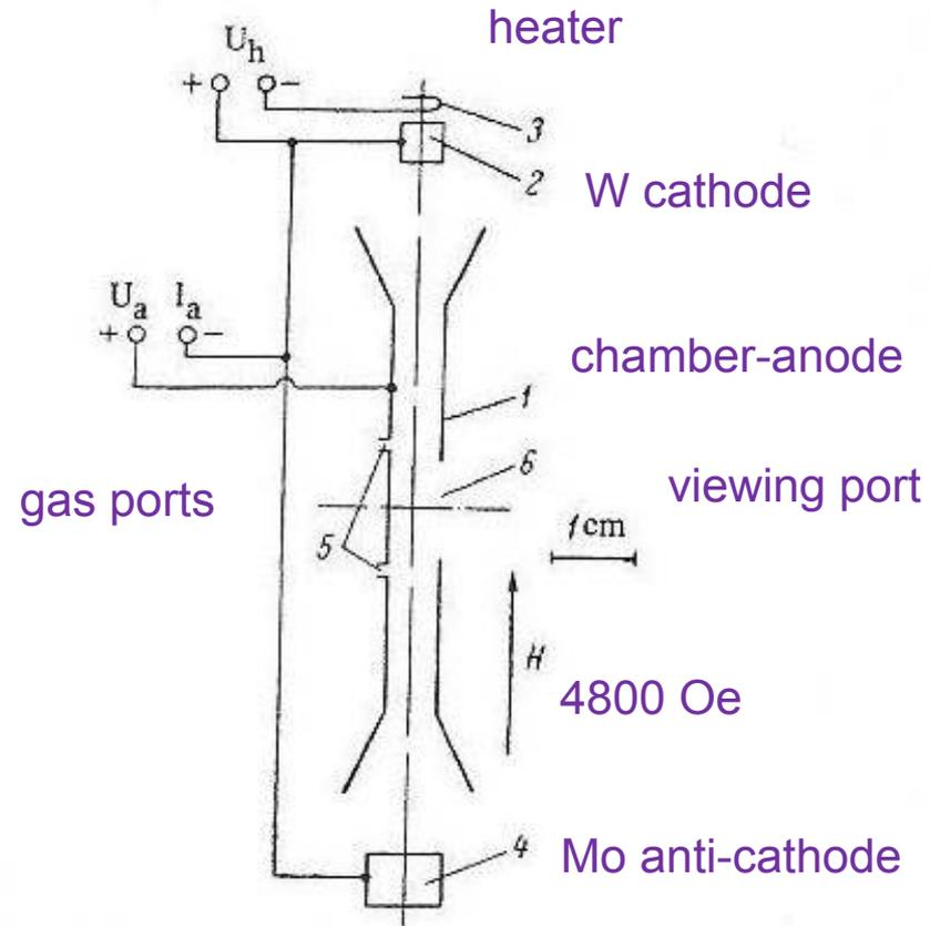
Fig. 1. Diagram of the multiply charged ion source.
