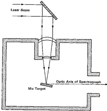
FIG. 1. Experimental arrangement for laser-produced plasma. The laser beam is about 2 cm in diameter. The target is inclined toward the spectrograph at an angle of about 5°.
