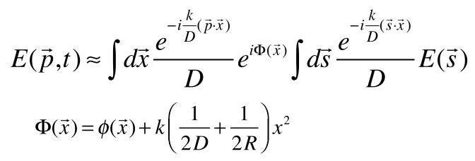
For an incoherent source, the intensity in the observer plane is an image of the source, convolved with the response of the screen to a point source.
