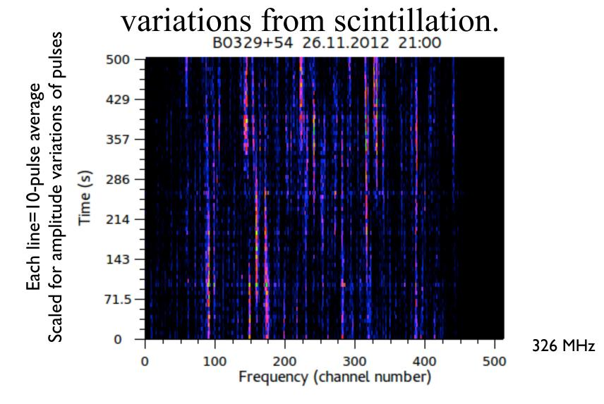
Selected strong scintillations in the dynamic spectrum provide accurate interferometer phases.
