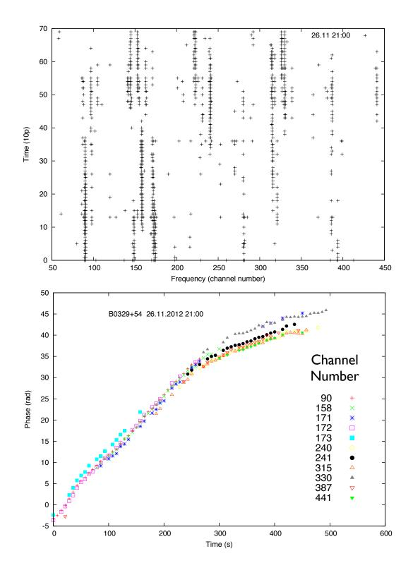
The variations of phase with time split the fringes in the delay/fringe-rate domain. This splitting decreases with increasing baseline length.
