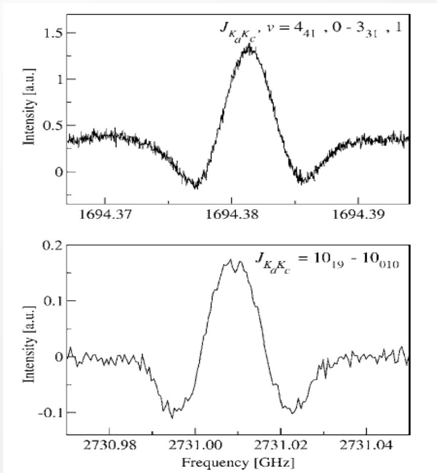
Spectra of ND<sub>2</sub>H (upper panel) and D<sub>2</sub>O (lower panel)
