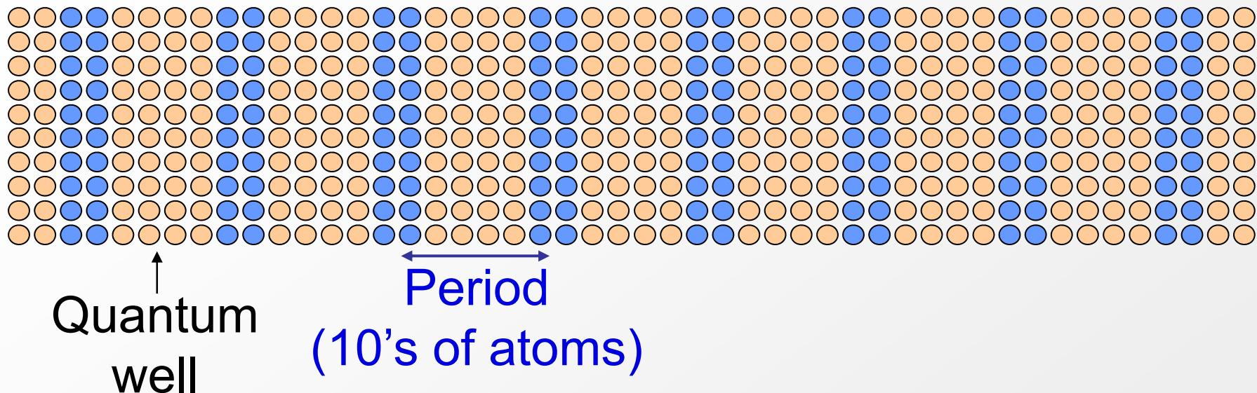
Chain of quantum wells forms a 1D periodic structure similar to a crystal lattice
